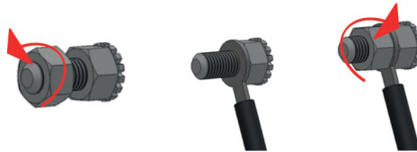
Figure 22. Connecting the unit to an electrical equalizing system.
